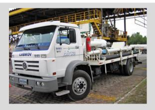
Hirsa has mobile calibration units for flow meters (tax appropriation and transfer of custody), LABMOV, which operate in the field, in the maintenance of equipment to ensure the compliance of flow measurement systems with the joint ANP / Inmetro ordinance, without interruption of operation.
